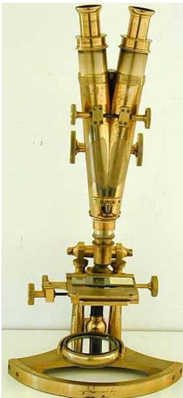
Other attempts were made, including a three part (achromatic?) prism assembly by Dancer. The Dancer method utilised two body tubes in a true “V” format, to split the light into two equal halves, so that each eyepiece receives the same amount of light from the objective. This gives a technically better (albeit more expensive) solution. The Dancer binocular prism method was registered No 4380 June 27<sup>th</sup> 1861. Compare this with the Wenham prism here.
